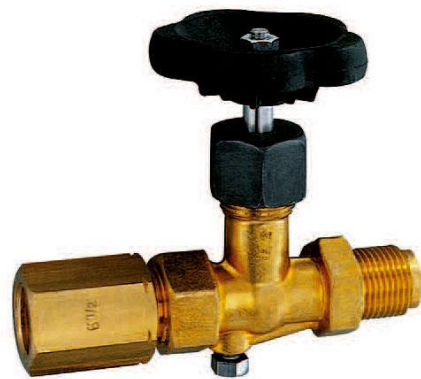
Shut-off valve per DIN 16270, LH-RH adjusting nut / male G ½, PN 250
