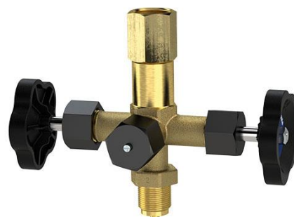
Shut-off valve with separately isolated test connection per DIN 16272, LH/RH union/male G ½, with test pivot M20 x 1.5, PN 400
